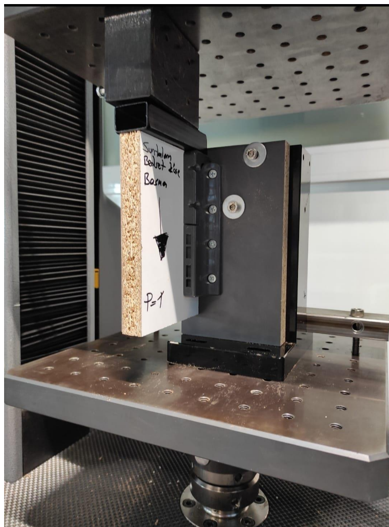
Figure 1. Compression test of chipboard module combined with Bedset Slide fixing apparatus.
