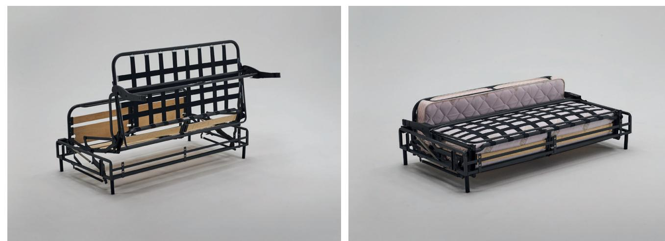
Conversion into a bed by only one movement without the necessity of removing seat and back cushions. A height of 32 cm, with 15 cm front border and 13 cm legs, allows a comfortable modern sofa with a seat height of 43 cm. Suitable for foam, fibre, or feather back cushions. Two independent orthopaedic wooden slatted sleeping decks for personal comfort either side of the bed. Mattresses available: pocket Spring (12 x 200cm), polilatex (11,5 x 200 cm) or foam (10/11 x 200 cm). Legs H 8 cm.
